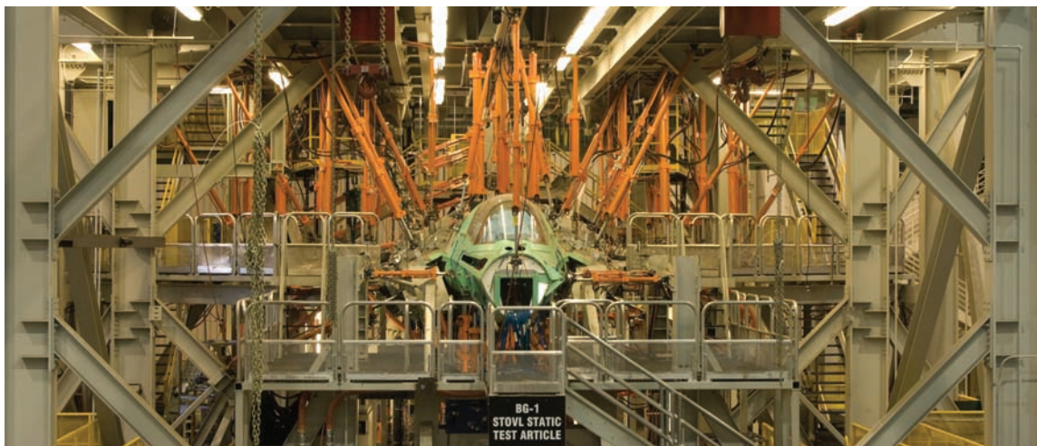
Measuring thousands of strain channels on F-35 Lightning II Joint Strike Fighter test article
