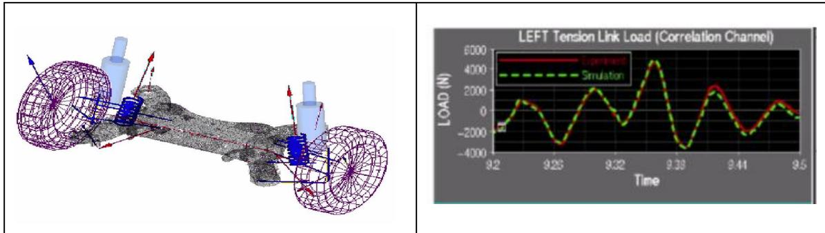
Figure 3. Virtual prototype of rear suspension
