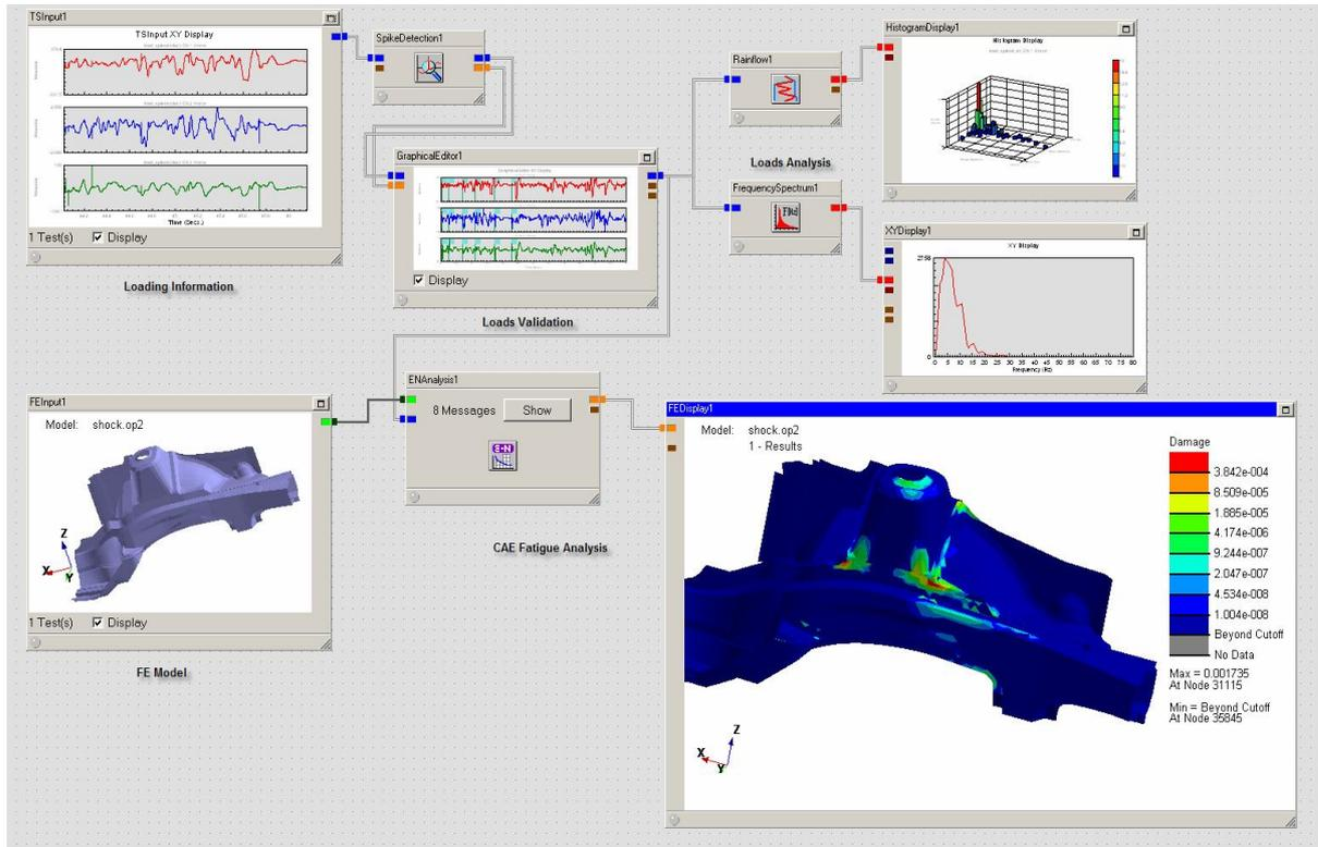
Figure 7. Test & CAE fatigue example analysis flow
