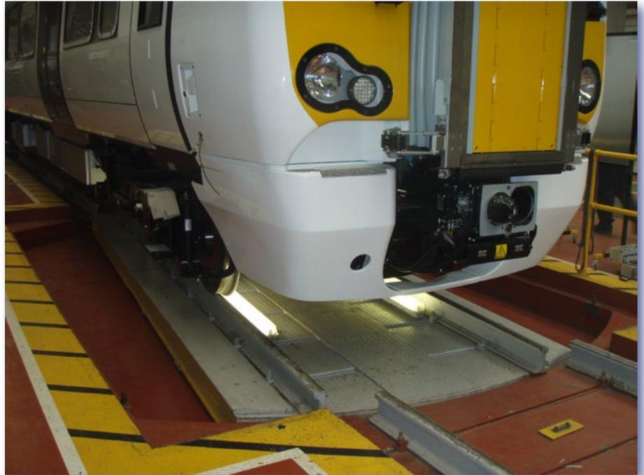
*The Bombardier Derby Test Facility Bogie Rotation rig. A new UK passenger train undergoing a bogie rotation test, allowing the design engineers to validate the resistance to rotation between the bogie and carbody.*
