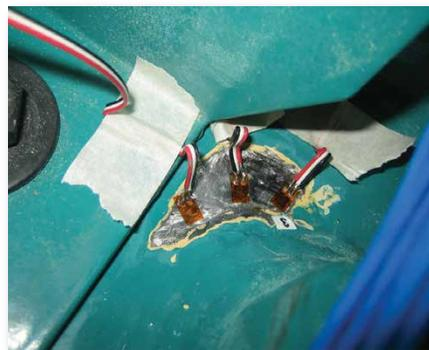
Strain gauges on bed frame
