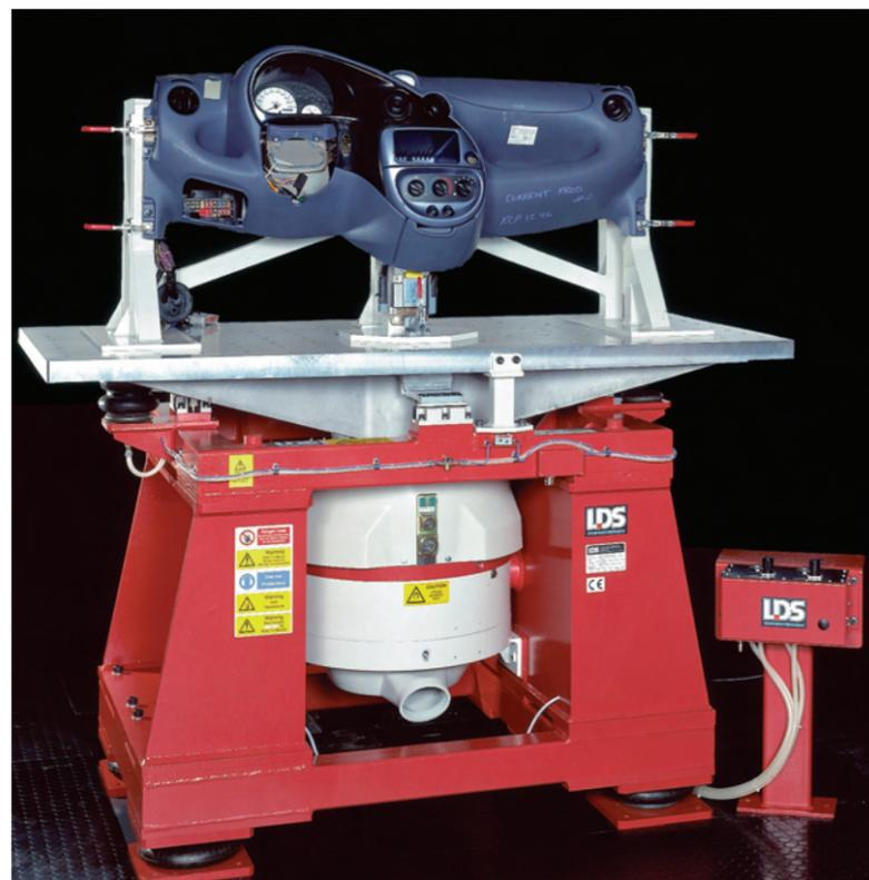
LEFT: Many components are signed-off with tests on electrodynamic shakers, but which test to use? (Image courtesy of LDS Test and Measurement.)
