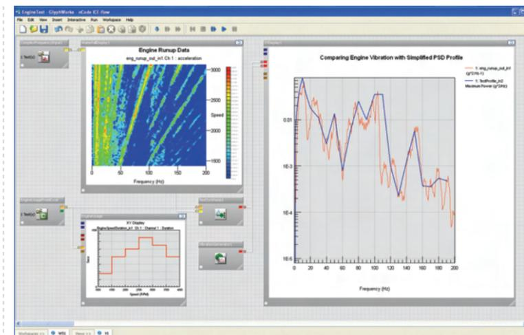
LEFT: A waterfall plot of engine vibration is combined with expected usage to create a representative vibration test
