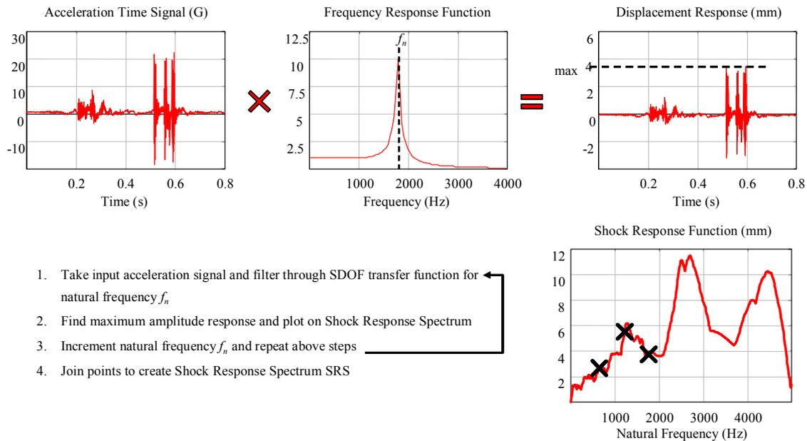
**Figure 2: Calculating the Shock Response Spectrum (SRS)**
