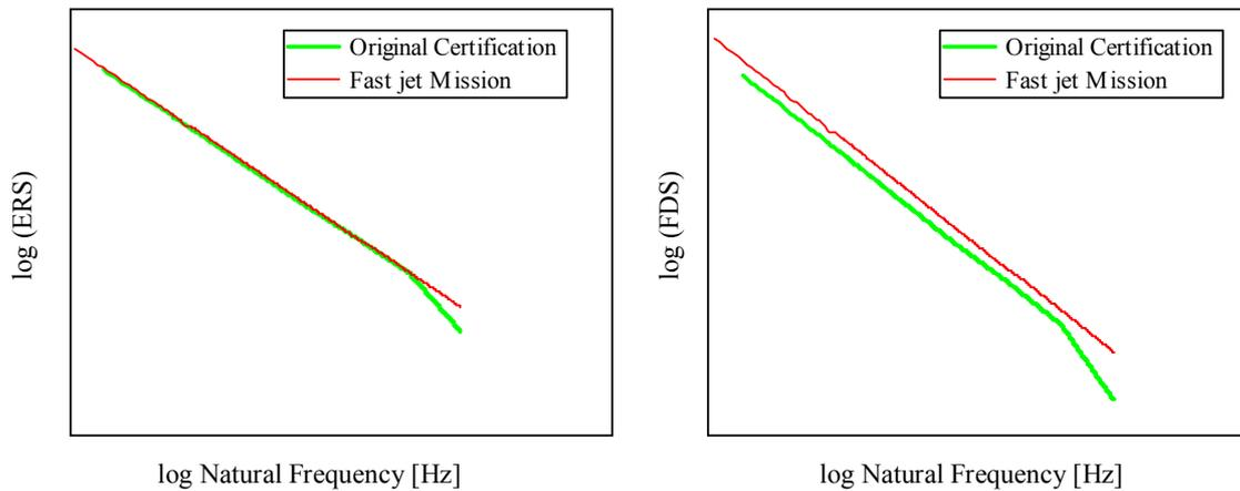
**Figure 7 Comparison between ERS and FDS of original certification test and fast jet design spectrum**
