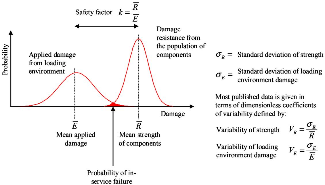
**Figure 5: Probability of in-service failure**
