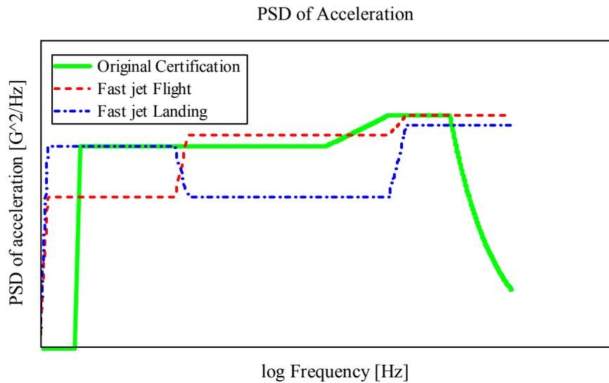
**Figure 6 Comparison between PSDs of original certification test and fast jet design spectrum**
