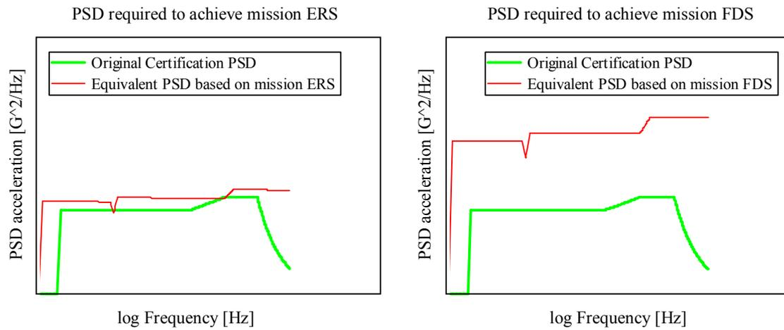
**Figure 8 Comparison between equivalent PSDs**
