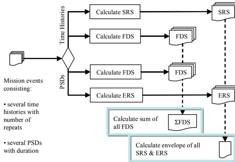
**Figure 3: Obtaining the Lifetime FDS and SRS**
