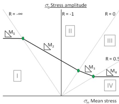
Figure 6 Haig diagram from [11] used for cycle mean stress correction
