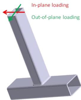
Figure 7 'T' specimen subjected to various ratios of in- and out-of-plane loading
