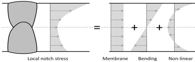
Figure 1 Local notch stress at a weld toe, comprising membrane, shell bending and non-linear stress peak
