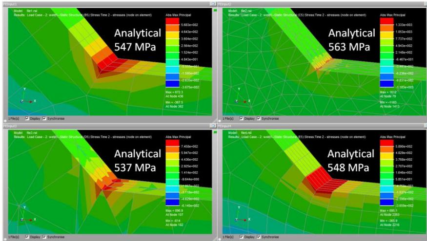
Figure 5 Investigation on mesh sensitivity to analytical extrapolated surface stresses
