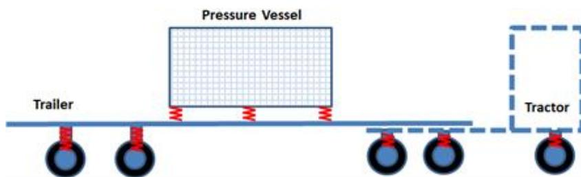
Figure 14 Schematic of the pressure vessel during road transportation
