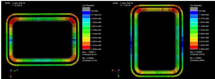
Figure 8 FEA-based fatigue analysis of 'T' coupon correctly identifying all initiation sites
