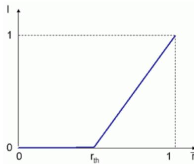
Figure 3 Interpolation function between membrane and bending SN curves
