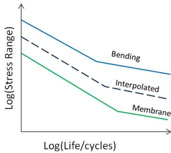
Figure 2 Interpolation between membrane and bending SN curves
