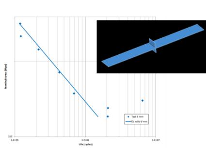
Figure 10 Comparison with TWI [12] NLC short attachment to both sides
