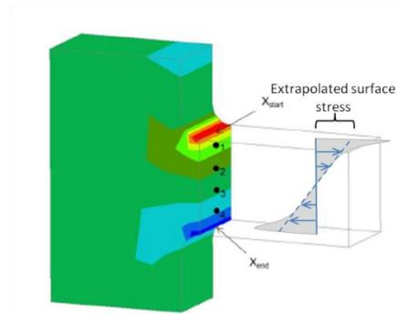
Figure 4 Through-thickness stress recovery with surface extrapolation
