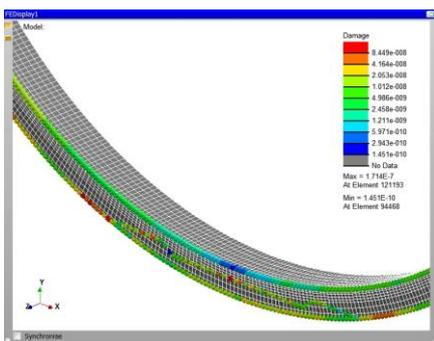
Figure 15: Weld seam damage plot
