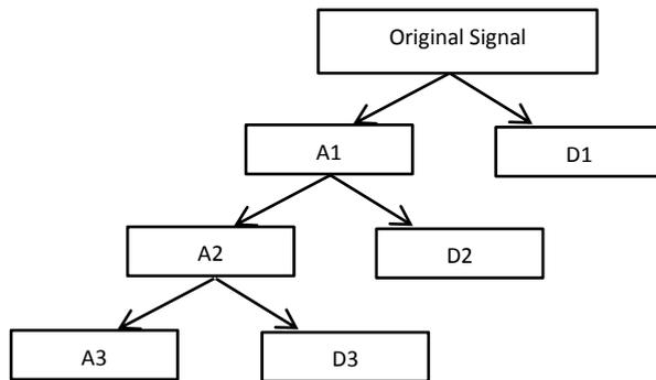
**Figure 1** – Structure of the DWT. The approximation and detail coefficients for level  $i$  are labeled  $A_i$  and  $D_i$  respectively. Note that for an  $n$  level DWT, the whole spectrum of the signal is captured with coefficients  $D_1, D_2, \dots, D_n, A_n$ .
