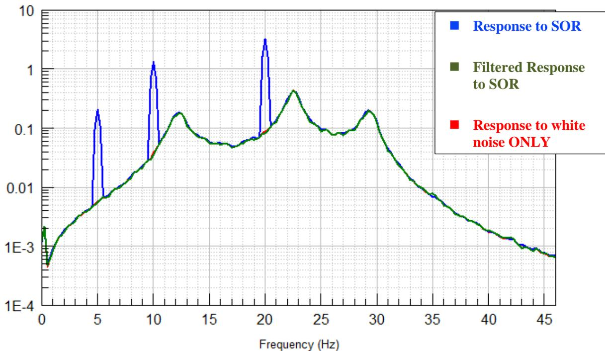
**Figure 5** – Application of the harmonic filter to the removal of three sine tones from a simulated response to a 3-DOF system (green). This response is compared to the response of the system to white noise excitation (red). It can be seen that the filtered response matches the response to white noise.
