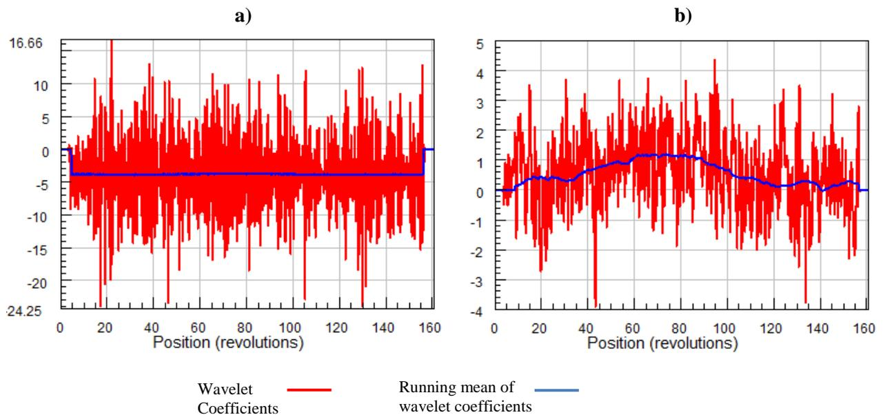
**Figure 4** – Wavelet coefficients of the relevant sub-bands for a helicopter signal containing harmonics and sampled at a condition that meets (11). Signals for two different events are shown a) rotor harmonics have largely constant amplitude, b) Rotor harmonics exhibit transients in amplitude.
