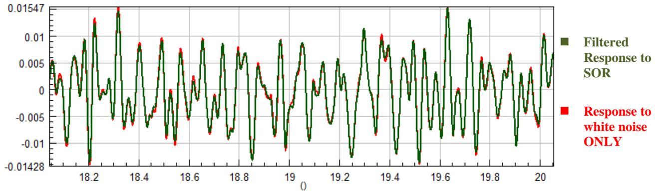
**Figure 6** – Time domain comparison of the 3-DOF system results. Only the filtered response (green) and the response to white noise are shown (red). It can be seen that even in the time domain, the filtering has very little distortion.
