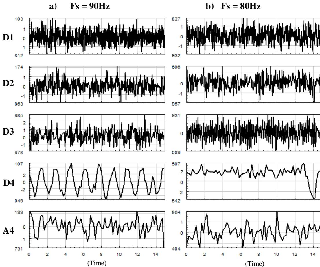
**Figure 2** – DWT down to 4 levels applied to two signals composed of white noise and a sine tone at 5 Hz. a) was sampled at 90 Hz, b) is sampled at 80 Hz and meets the condition for a harmonic appearing as offset. Note how the coefficients in D4 are periodic in a), while an offset is evident in b).
