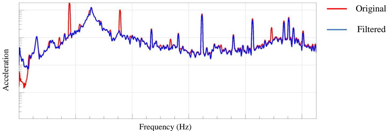
**Figure 7** – Result of applying the filter to all of the nodes to remove all harmonics of the main rotor of a helicopter. This example shows how this method removes the harmonics without interfering with the underlying dynamics. Note that the harmonics that are left are not harmonics of the main rotor.
