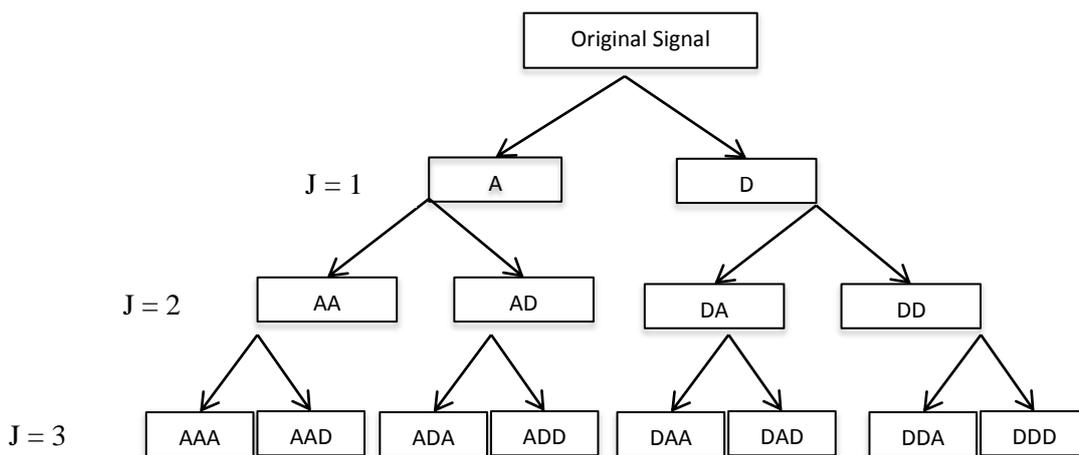
**Figure 3** – Filter bank structure of the Wavelet Packet Decomposition (WPD).
