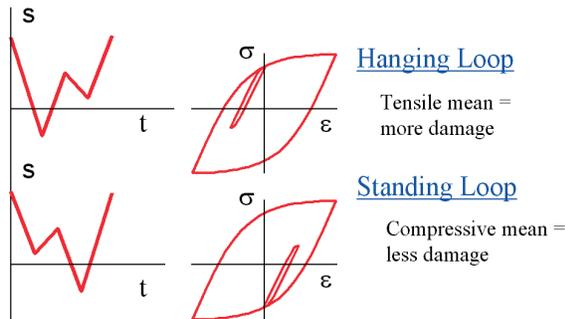
**Figure 7** Illustration showing the effect of cycle sequence
