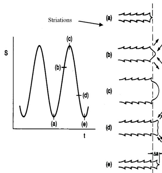
**Figure 5** Illustration of Stage II crack growth
