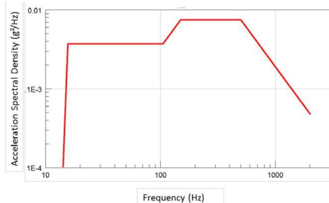
Figure 4: The excitation PSD used for Gaussian and non-Gaussian loadings.
