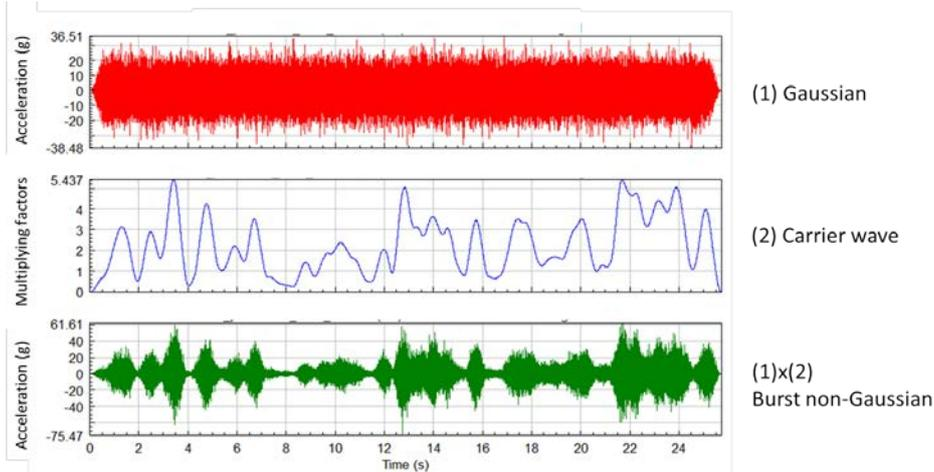
Figure 2: Construction of a burst non-Gaussian signal
