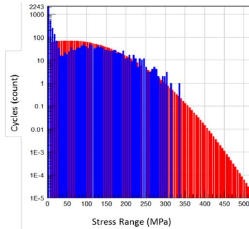
Figure 11: Rainflow histograms from time domain (blue) and spectral domain (red) for a 50 second exposure duration.
