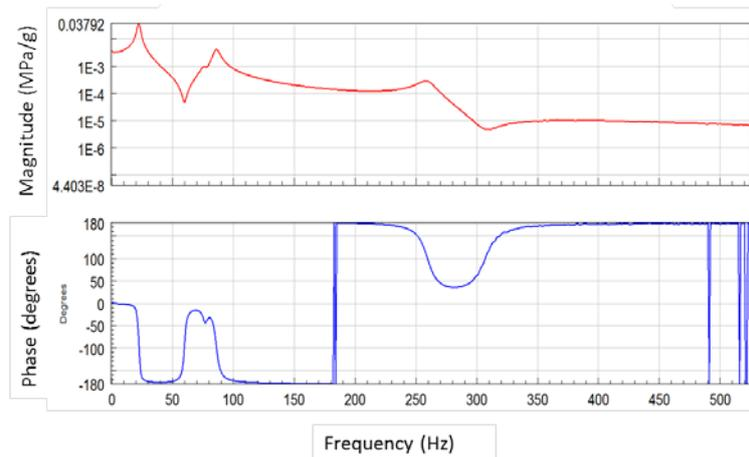
Figure 7: Stress FRF obtained at a critical node (3100).
