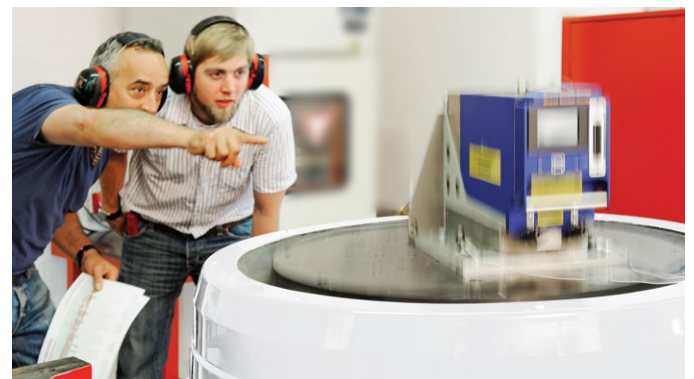
Brüel & Kjær LDS shaker system from HBM
