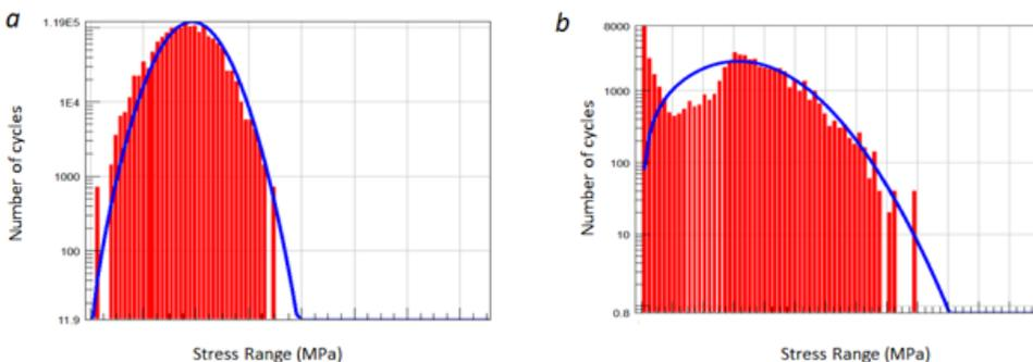
Fig. 5: Comparison between rainflow cycles using the time-domain (red) and spectral (blue) approaches.
