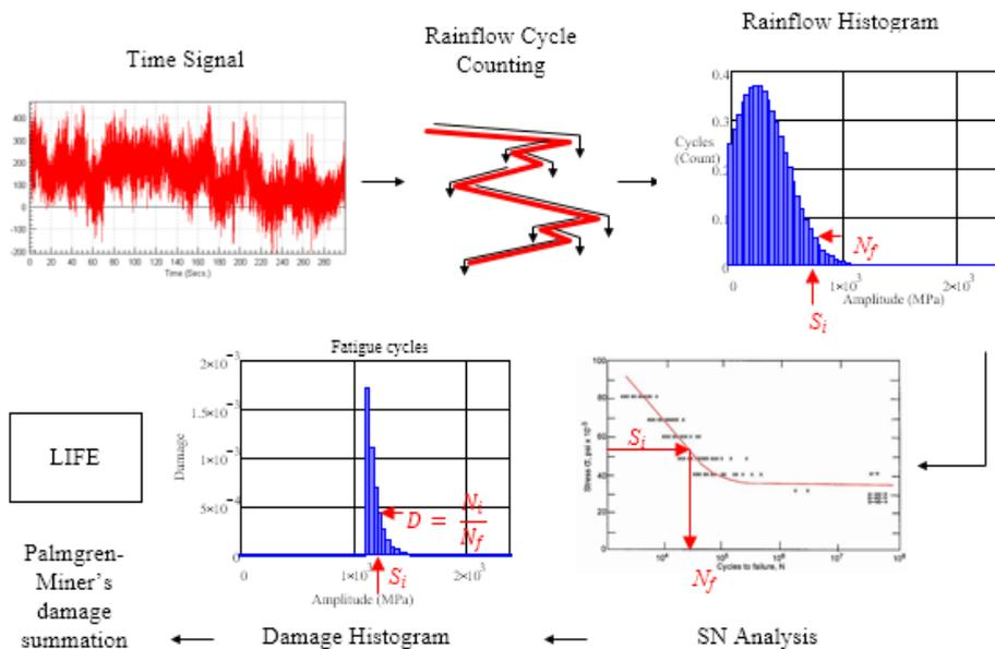
**Fig 1: Time-domain fatigue analysis**
